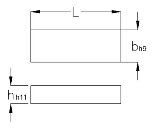
b = 6 h = 6 L = 20 Tolerance b = 0.030 Tolerance h = 0.075
